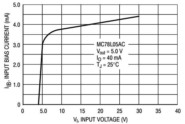
**Figure 6. Input Bias Current versus Input Voltage**
