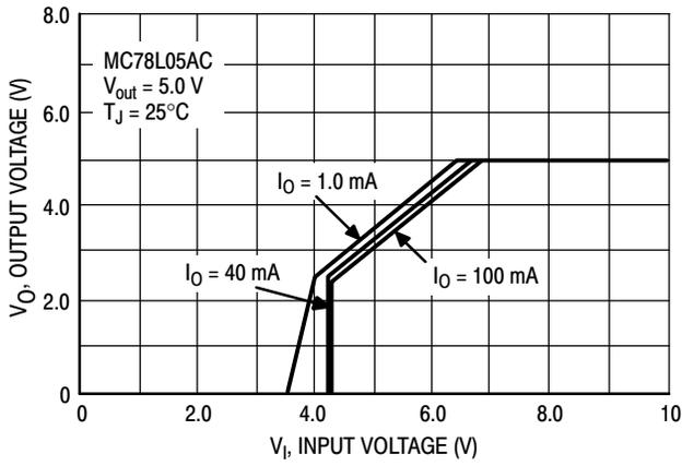
**Figure 3. Dropout Characteristics**
