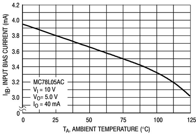
**Figure 5. Input Bias Current versus Ambient Temperature**
